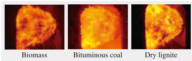
Fig. 8—DS-T Burner Flames for Different Fuels (Air Combustion).
